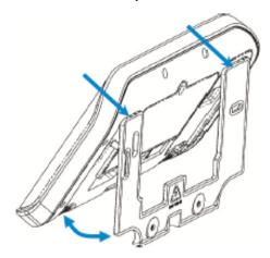
**NOTE**: Ensure the screw on the underside of the panel is loosened enough so that the wall bracket clears the screw head; if not the panel may not fit flush against the wall. Then retighten the screw to ensure a secure fit.
