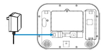
Connect the power supply to receptacle.
