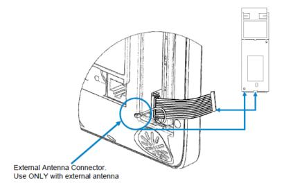
Connect an external antenna to the antenna connector on the back of the Côr<sup>™</sup> panel. To obtain maximum signal strength the external antenna must be fully extended. Re-check signal strength following steps in section 7.3.
