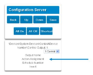
6. Press the drop down action menu and select the action you want to control the output. The output will now be controlled by the state of the selected action.
