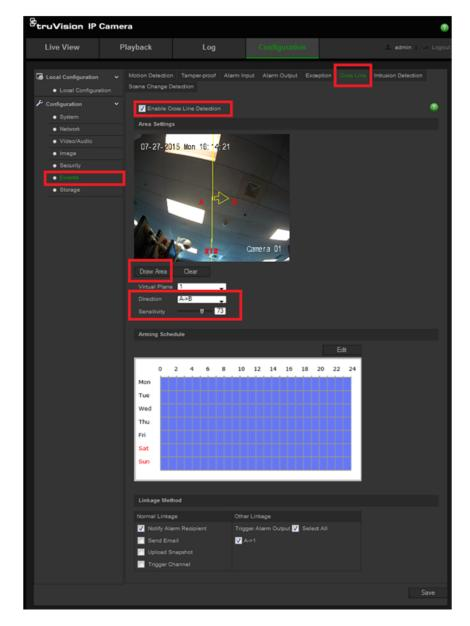
Select **Draw Area** and click and drag in the video to create a vertical line. This should be near the door. The arrow (set by the direction option) needs to be pointed into the room. See the diagram above. Make sure the  $A \rightarrow 1$  is checked and the *Day/Hour Grid* will appear in *blue* color.
