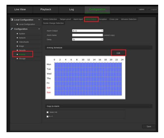
The Day/Hour Grid will appear in blue color as shown above. This will ensure that the alarm output will trip whenever there is motion.
