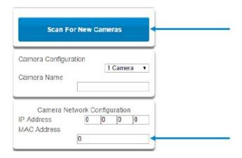
Make sure the MAC ID that is automatically populated in the MAC Address field matches the MAC Address printed on the back of the camera. If not, change in the MAC Address to the one listed on the back of the Camera.
