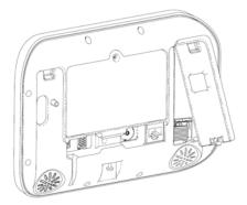
Locate the 10-pin lead inside the Côr™ and connect this to the radio module.
