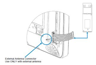
Insert the whole radio module in to the Côr™ taking care not to crimp any cables. Replace the cover on the Côr™
