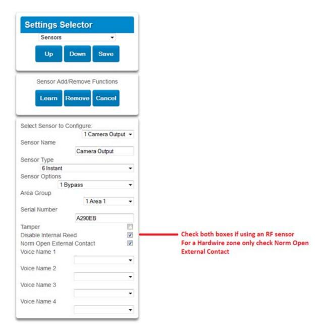
For the purpose of this demo the zone will be an instant perimeter. This can be set to whatever zone type/option you desire. To make it work like a traditional interior follower, set the **Sensor Type** as Follower and **Sensor Option** as *Bypass Stay*.
