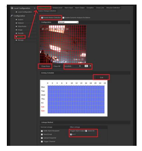
Check **Enable Motion Detection**. Select **Start Draw**. Drag inside the video image to create the red grid. The red grid is the area that the camera will look for motion. Adjust the **Sensitivity** as needed. The light bulb next to Sensitivity will light up when the camera detects motion. Make sure the **Trigger Alarm Output > A \rightarrow 1** is checked. Ensure that the Day/Hour Grid is a blue color as shown above. This will ensure that the camera will detect motion 24/7.
