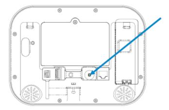
Move the panel or the antenna to another location if the signal is still too low. Place the external antenna to optimize signal strength.
