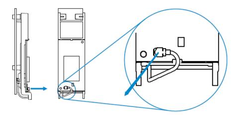
Gently pull retaining clips outwards and remove the rear circuit board. This is the internal antenna which will no longer be needed.
