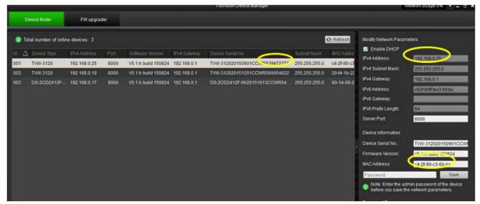
Once you have selected the camera, the parameters of that camera will be displayed in the fields to the right of the screen. Write down the *IPv4 Address* and *MAC Address* associated with the camera.
