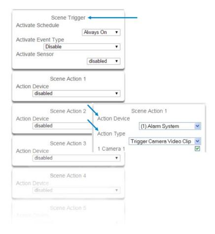
Select Action Device (1) Alarm System. This enables another drop down menu for Action Type. Choose the Action Type "Trigger Camera Video Clip", then the cameras you wish to record a video clip when the event is triggered.
